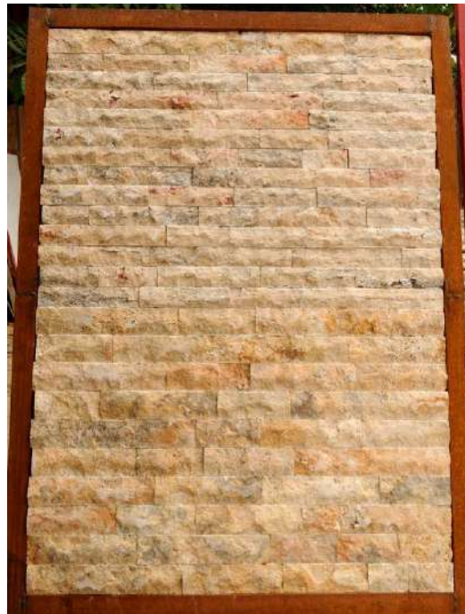
Figure 14. Travertine half processed pellets (stone tile) from Lipkovo deposit [URBANTEK-Radovis]
